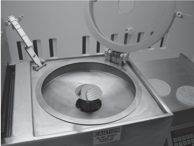
FIGURE 2.3 A bare silicon wafer mounted on a vacuum chuck and ready to be coated with photoresist (Courtesy of Center for Hierarchical Manufacturing, University of Massachusetts, Amherst.)
